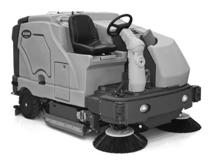
The Advance SC8000<sup>™</sup> rider scrubber is the definition of innovative and optimized design. This maneuverable front steer scrubber houses the widest cylindrical scrub deck in its class. This deck's dual counter-rotating cylindrical brushes are capable of sweeping and scrubbing in a single pass. DustGuard<sup>™</sup> suppresses and controls dust using a "fog" at the side broom. Using Advance's One-Touch<sup>™</sup>, the entire scrub system is activated simply by the press of a button.
