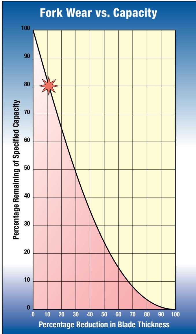
**This chart shows how fork wear reduces truck capacity. ANSI standards require that each fork be rated at least half the capacity of the truck at the rated load center distance as shown on the truck nameplate.**
