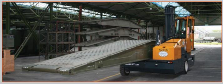
Two C10,00SL Combilifts have been drafted in by the UK Defence Storage and Distribution Agency (DSDA) to work at its vehicle and equipment storage facility due to the extreme maneuverability and versatility they offer for handling a very specific and problematic type of load – components for assembling tank and infantry bridging.
